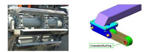
• **Sprocket:** The hardworking sprockets, rollers and bushings (embedded within the rollers) are machine finished to high precision and subsequently induction hardened. This reduces the need for frequent replacement and costly maintenance down time. Rollers are travelling on a strip of wear resistant steel, preventing them from prematurely wearing down to the pontoons.
