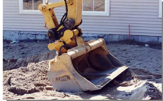
★ PROVIDES POSITIVE, POWERFUL TILTING - 45deg IN EITHER DIRECTION FOR SLOPE GRADING, BACKFILLING, DITCH CLEANING, CUTTING SLOPED TRENCH, SHAVING TRENCH EDGES etc..
